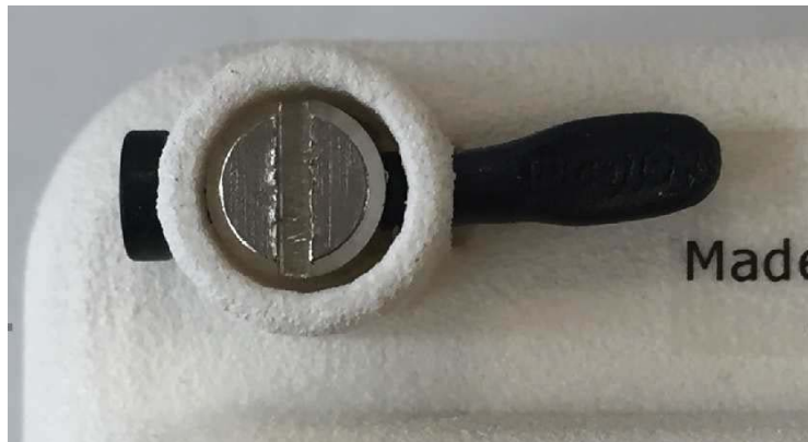
Figure 2: Meter with Certification PIN seal
